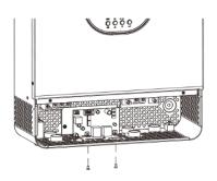
**Step 3:** Remove two screws as below chart and remove 2-pin and 14-pin cables. Take out the board under the communication boards.
