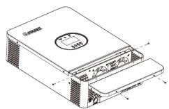
Step 2: Remove WiFi/GPRS communication board and CAN/RS485 communication board by unscrewing screws as below chart.
