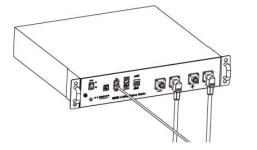
**Note:** if choosing lithium battery, make sure to connect the BMS communication cable between the battery and the inverter. You need to choose battery type as "lithium battery"
