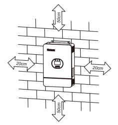
Install the unit by screwing three screws. It's recommended to use M4 or M5 screws.
