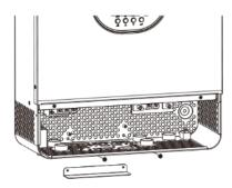
Step 5: Install new parallel board with 2 screws tightly.
