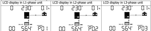
Step 4: Switch on all AC breakers of Line wires in AC input. If AC connection is detected and three phases are matched with unit setting, they will work normally. Otherwise, if will display warning 15/16 and they will not work in the line mode.
