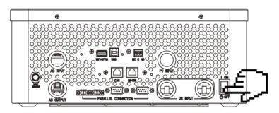
Once the unit has been properly installed and the batteries are connected well, simply press On/Off switch (located on the button of the case) to turn on the unit.
