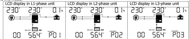
Step 5: If there is no more fault alarm, the system to support 3-phase equipment is completely installed. Step 6: Please switch on all breakers of Line wires in load side. This system will start to provide power to the load.
