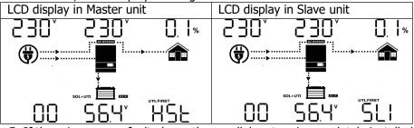
Step 5: If there is no more fault alarm, the parallel system is completely installed. Step 6: Please switch on all breakers of Line wires in load side. This system will start to provide power to the load.
