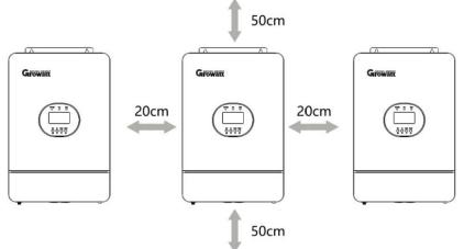
**NOTE:** For proper air circulation to dissipate heat, allow a clearance of approx. 20cm to the side and approx. 50 cm above and below the unit. Be sure to install each unit in the same level.
