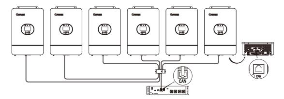
Note: If inverters parallel as 3 phase system, only need to connect L1-Phase inverters with lithium battery to communicat with BMS.When inverters on L1-Phase are more than 2 units, it would need an extra RS485/CAN HUB to converge inverters on L1-Phase to connect with lithium battery to communicate with BMS.
