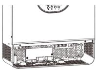
Step 6: Re-connect 2-pin and 14-pin to original position.
